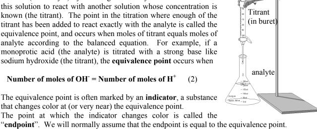
There are many types of titrations. In this lab you will be performing an acid base titration.
