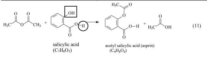
You can perform a colorimetric test to determine if there is any salicylic acid left in your sample. Addition of  $FeCl_3$  to phenols results in the formation of a colored complex. The OH (shown in the box above) attached directly to the benzene ring is called a phenol. This type of OH is different from the OH where the H is circled above or an OH of an alcohol. Addition of  $FeCl_3$  to salicylic acid will result in the formation of a deeply purple colored complex.
