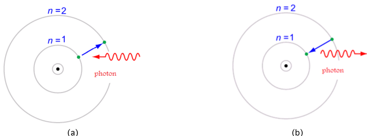
Figure 4a shows an atom in its ground state, with the electron (green dot) moving from level 1 to level 2 by absorbing energy from an incoming photon. Figure 4b shows an atom in an excited state emitting a photon as its electron moves to a lower energy level. Only two levels ( n=1 , n=2 ) are shown
