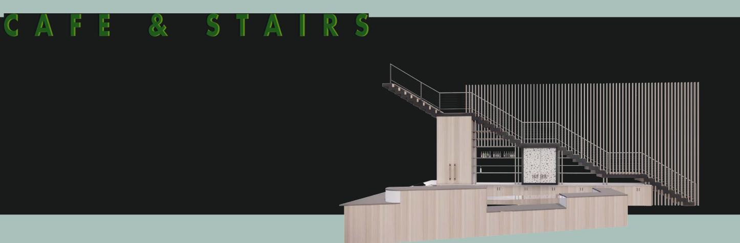
WOOD TREADS STEEL STRINGER STEEL RISERS 2" WOOD HANDRAILS BACK-LIT SHELVES
